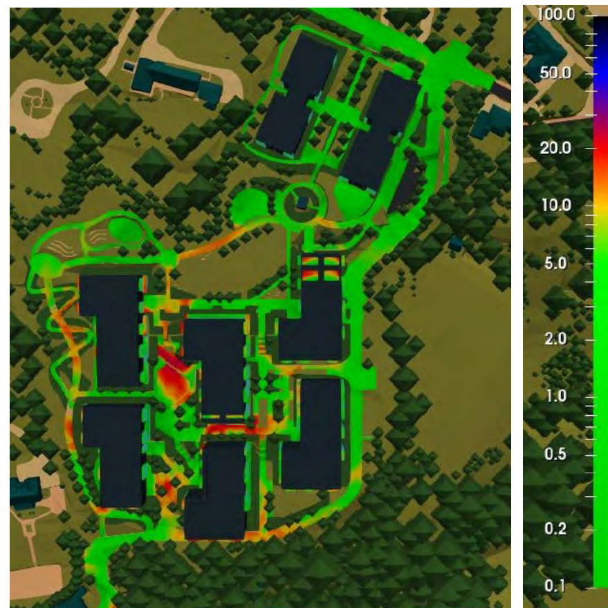
Sitting Comfort Criterion: Ground Amenities from Barrington Cabinteely Wind Study - Wind Microclimate Study by IES Green colour indicates comfortable zones.
