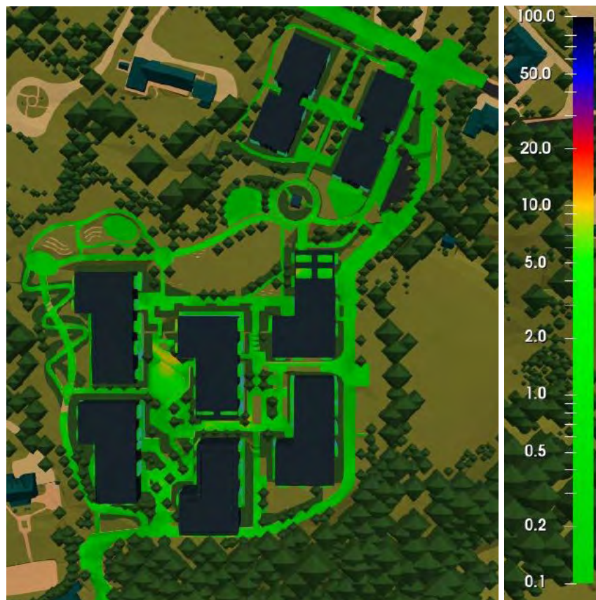
Standing Comfort Criterion: Ground Amenities from Barrington Cabinteely Wind Study - Wind Microclimate Study by IES Green colour indicates comfortable zones.
